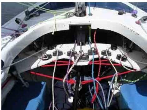
Compared to the 2 ropes in the 2.3, you get 18 of them in the 2.4 including the seat angle adjustment line! There are also 4 shrouds which can be tweaked at your leisure although these are admittedly usually left alone once at the correct tension. 18 ?! I hear you say! Well, in case you are wondering what so many control lines could possibly be meant for, here is a list:
